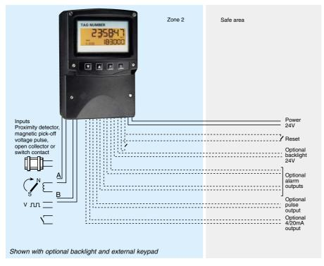
The BA364ND is a Type nL certified multi-function instrument which may be programmed to perform a host of counting and timing functions. Easy to use menus allow the instrument to be configured as a counter, timer, tachometer or as a clock. Both of the inputs will operate from 2-wire proximity detectors, switch contacts, magnetic pick-offs, open collectors or voltage pulses. Optional alarm/control outputs further extend the many applications.
